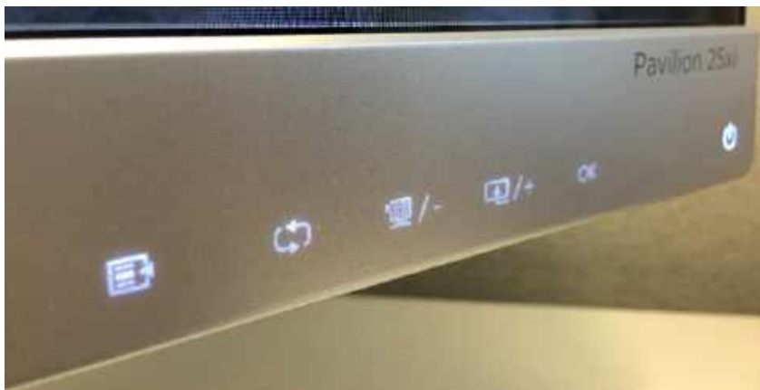
Figure 12 Tactilely Discernible – Failing Example
